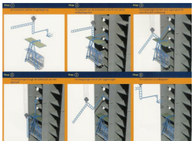
Figure 6: A mechanised panel assembly system developed by BALLAST NEDAM. 'The panels are installed using a flying scaffold suspended from a tilting arm. The tower crane uses this tilting arm to pick up the flying scaffold. The tilting arm's grab is positioned above the floor where installation will take place. Using its own weight, the flying
